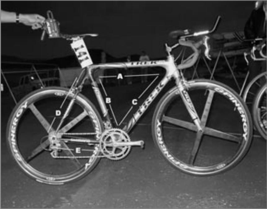
**PHOTO 1.1** *Standard double diamond frame design*
