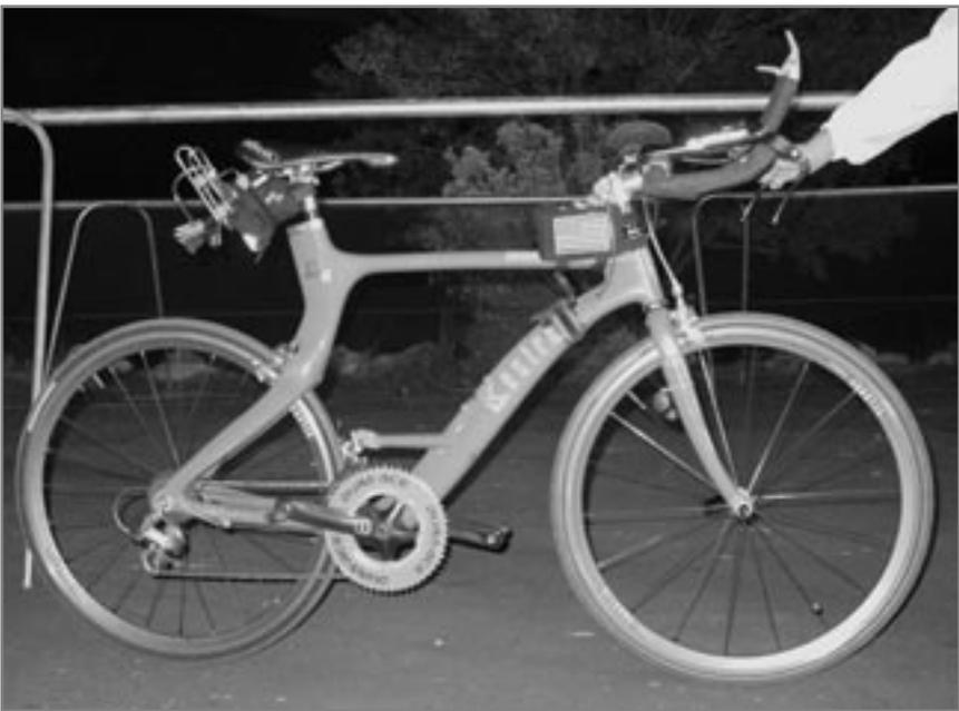
**PHOTO 1.2** *The Kestrel KM40 is a carbon fiber bike with no seat tube.*
