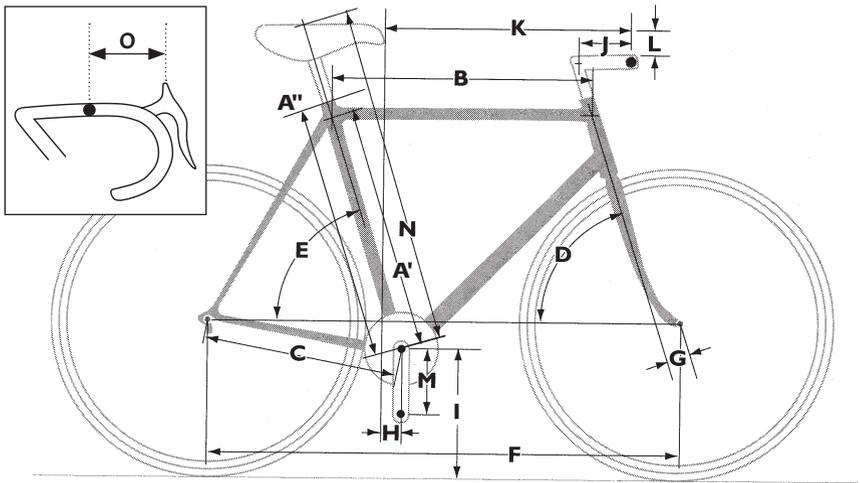
**FIGURE 1.3** Road Bike Measurements
